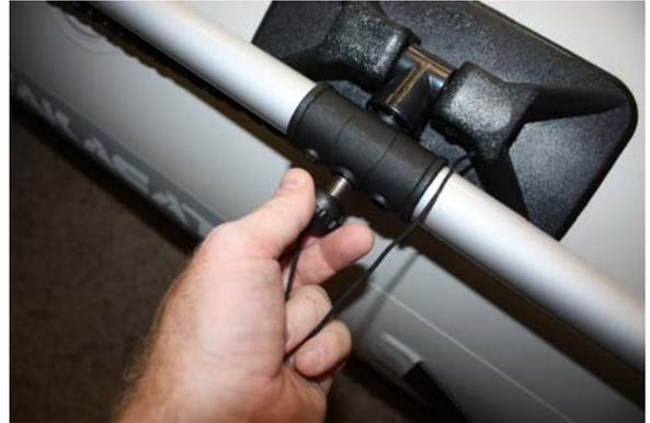
11. Assemble each oar and install. Be sure to attach retaining nut to prevent losing oars when in use.
