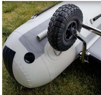
12. If you opted for the Quick Release Beach Wheels, install them now in the down position. When in the down position, the wheels provide enough height to mount a 15" short shaft outboard in the upright position.
