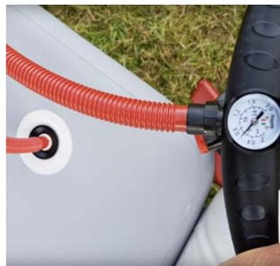
9. Inflate the floor to 10 psi. While inflating be sure to pause and walk on the floor to push it into place. Don't forget to activate the check valve by pressing down on the center pin and turning it 1/4 turn in either direction, If it is popped up, it won't let any air escape.
