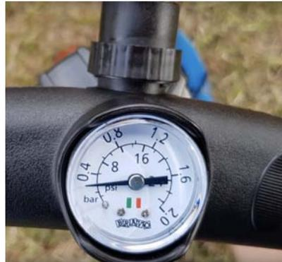
2. Locate the inflator valve at the rear of the hulls and inflate to 3 psi with the included hand pump or optional electric pump.
