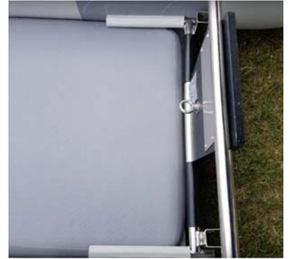
7. Unroll the inflatable floor and insert it into its position. There is no need to get it perfectly under each hull tube, but the rear of the floor should be flush with the Lower Transom Bar.
