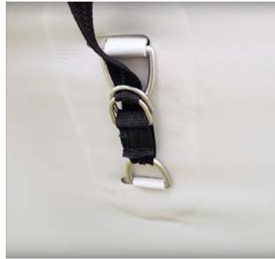
8. Insert D-Rings, on the bottom of the air deck floor, through the slots in the boat floor fabric layer.
