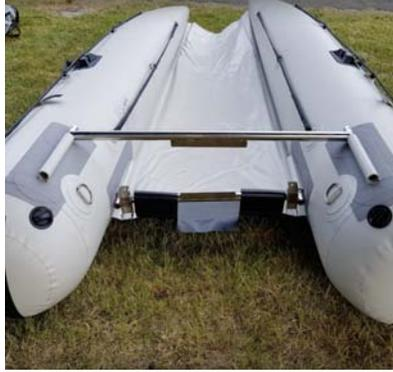
4. From the front, insert the upper transom bar into the upper set of tubes on the boat hulls. The stainless tab should be facing down when installed properly.
